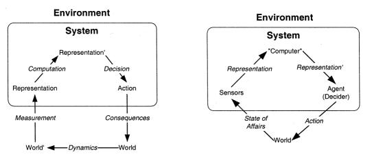
Fig. 6. Control system with computation: (left) functional and (right) structural.
