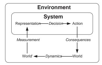
Figure 1: Functional view of a control system.
