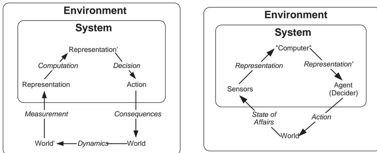
Figure 5: Control system with computation.
